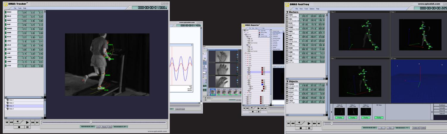
Spica Technology Corporation's 3D Digital Motion Analysis System – DMAS7™, supports 3D-6DOF Real Time and Automatic tracking with autolabeling to subpixel accuracy, including simultaneous recording of synchronized video, and offers users a choice of either static or dynamic calibration.
