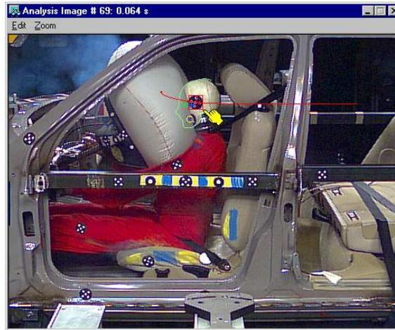
The FalCon **MovXact** module allows you to precisely analyze image sequences with the methods of 2D image measurement technology.
