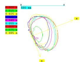
The analysis program **eXtra MovBag** offers automatic measurements of airbag outlines as contour graphs = f(t).
