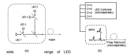
Figure 1. (a) Schematic diagram of a Mightex WFC-series multi-wavelength fiber coupled LED source; (b) Schematic diagram showing a WFC with a fiber patchcord (sold separately), powered by a Mightex multi-channel LED controller (sold separately),.
