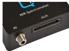
The Qred includes a new auxiliary connector for analog and digital I/O, communication interfaces and power supply (if USB is not used). The 8 digital channels can be configured as trigger input, shutter or flash lamp control, process control or general purpose I/O pins.
