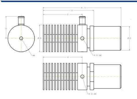
Installation Drawing for 22-mm LED Collimator, Type-A
