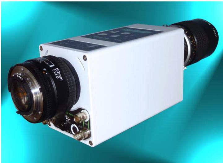
The UVi is easily programmed by its integral menu driven LCD display/control panel or via its USB interface and software to synchronize to an external TTL or video signal; offering multiple, digitally programmed gain, delays and exposures (from 10ns in 10ns steps) and at framing rates up to 10M fps in burst mode.
