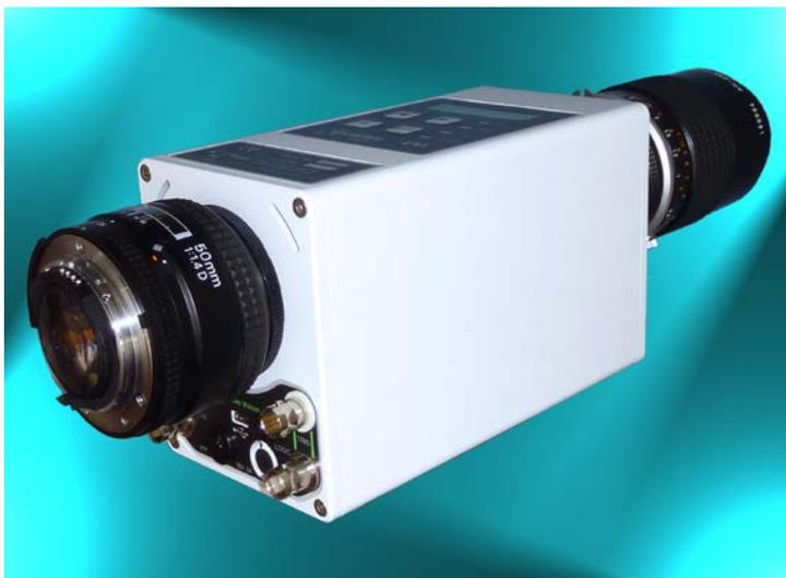
The UVi is easily programmed by its integral menu driven LCD display/control panel or via its USB interface and software to synchronize to an external TTL or video signal; offering multiple, digitally programmed gain, delays and exposures (> 10ns in 10ns steps) and at framing rates up to 10M fps in burst mode.
