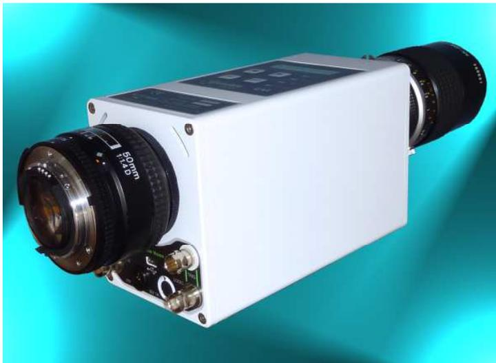
The UVi is easily programmed by its integral menu driven LCD display/control panel or via its USB interface and software to synchronize to an external TTL or video signal; offering multiple, digitally programmed gain, delays and exposures (> 100ns in 10ns steps) and at framing rates up to 10M fps in burst mode.
