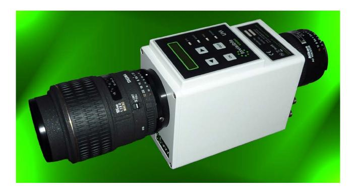
The UVi is easily programmed by its integral menu driven LCD display/control panel or via its USB interface and software to synchronize to an external TTL or video signal; offering multiple, digitally programmed gain, delays and exposures (> 10ns in 10ns steps) at input trigger rates to > 100,000 per second and up to 20,000,000 per second in burst mode.
