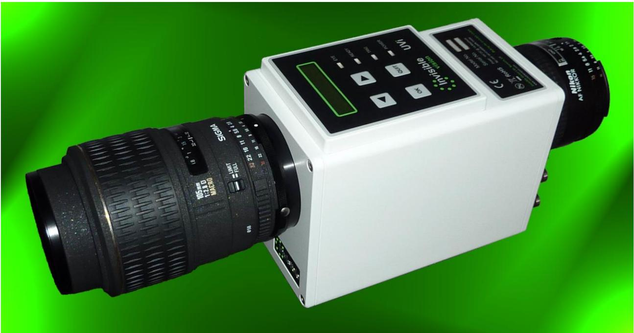
The UVi is easily programmed by its integral menu driven LCD display/control panel or via its USB interface and software to synchronize to an external TTL or video signal; offering multiple, digitally programmed gain, delays and exposures (> 10ns in 10ns steps) at input trigger rates to > 100,000 per second and up to 20,000,000 per second in burst mode.
