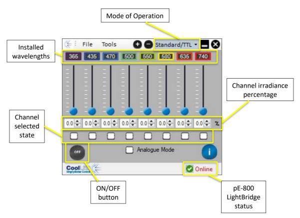
The LightBridge allows the full control of the pE-800. Any of the eight installed channels can be operated at the same time.
