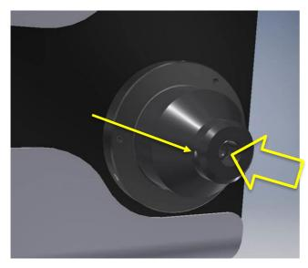
Remove the protective caps from the light guide and insert one end fully into the Light Source. Ensure that the grub screw is fully loosened to avoid any obstruction.
