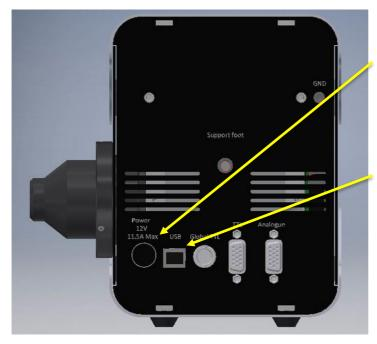
Insert the power supply connector into the Light Source. Ensure that the connector is correctly oriented, with the flat of the connector casing facing up.
