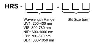
For example, HRS-VIS-010 is a spectrometer with a wavelength range of 390-780nm and a 10 μm slit size.
