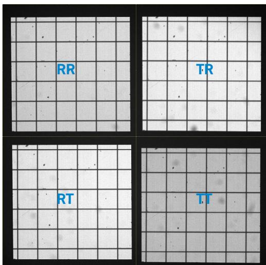
When using long pass dichroic mirrors, the four images correspond to the following channels in order of descending wavelength:
