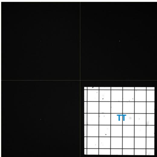
5. Remove the magnetic door cover and insert the first calibration cube into the position labelled Horizontal Split - Cube 1, which will generate your second image. This is reflected by the first filter cube, and transmitted by the second, hence the nomenclature **RT**.
