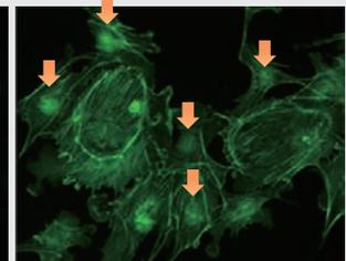
DAPI fluorescence leaks into the EGFP detection channel and causes artifact shapes of the nucleus in EGFP image. (Images are shown in pseudo-color.)
