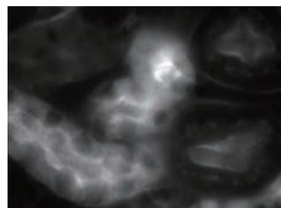
MAICO® detects fluorescence in the objective focal plane only, so high contrast optical sectioning images can be acquired.
