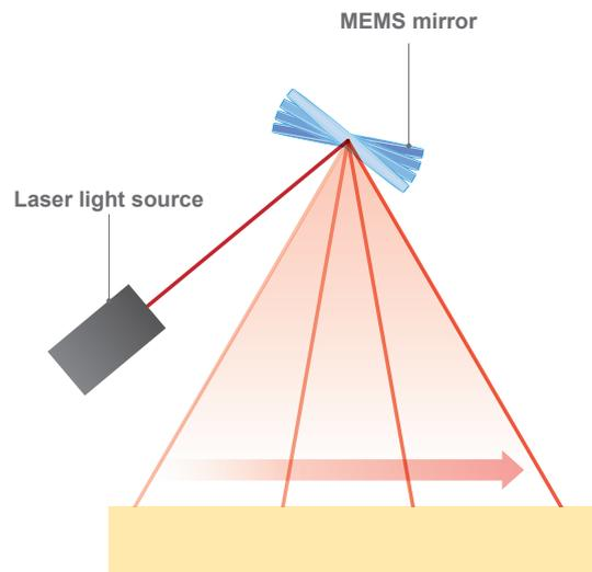
A light spot is scanned at 29 kHz resonant frequency.
