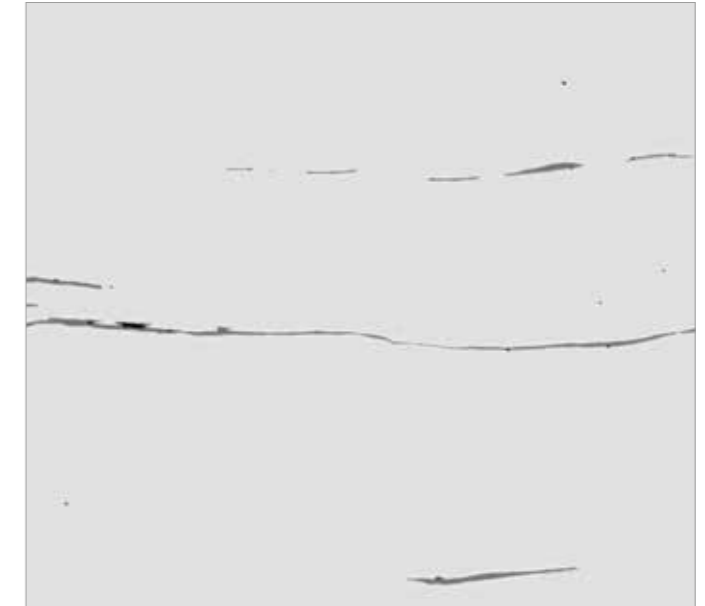
Non-metallic inclusions in steel Microscope: ZEISS Axio Imager.Z2m Objective: EC Epiplan-NEOFLUAR 10x/0.25 Camera: ZEISS AxioCam MRC
