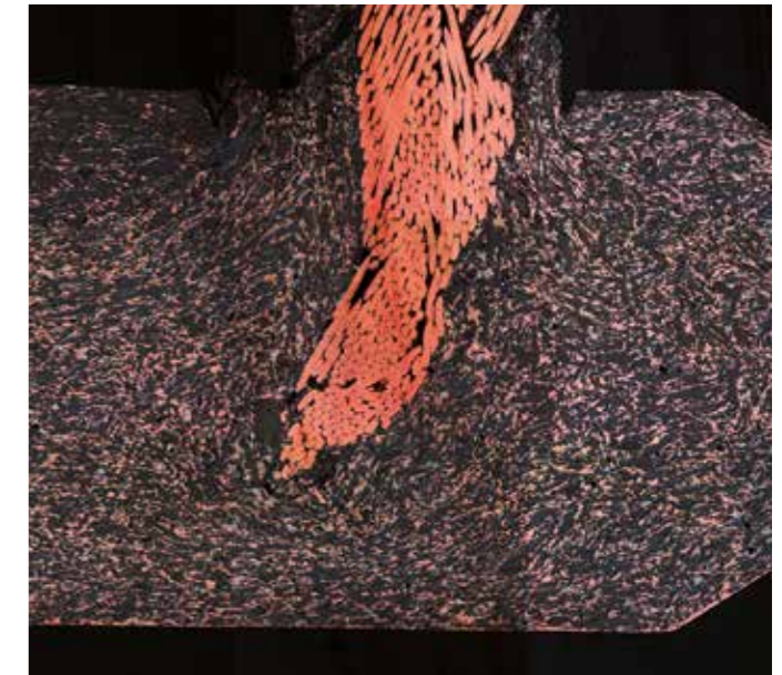
Carbon brush: extensive views of structural homogeneity; distribution of conductive phases such as Cu particles and hard phases; visualization of manufacturing effects
